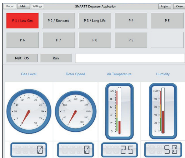
Picture 7. Operator screen
